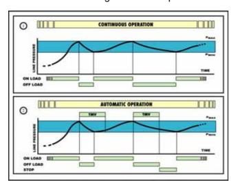
In "Continuous" operation the compressor delivers air within а maximum/minimum pressure range. When reaching the maximum pressure the intake valve closes. The compressor runs "off-load" and is decompressed to 2 bar to reduce the energy absorption. decreases When the pressure and the minimum reaches value. the compressor goes back to "load" and starts delivering air instantly.
